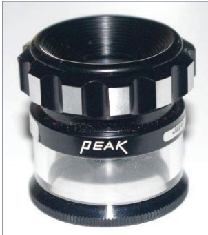
Eye loops were used until the 1990s to check PCB artwork for manufacturing suitability.
