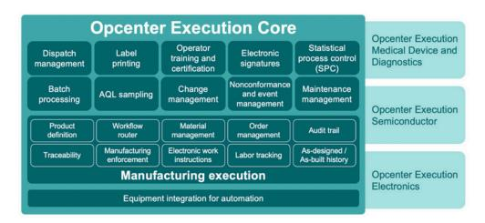
The modular architecture of Opcenter Execution Core includes advanced capabilities for comprehensive management of production, quality, traceability, and equipment integration. It serves as a scalable foundation for vertical solutions like Opcenter Execution for Medical Device and Diagnostics, Semiconductor, and Electronics.
