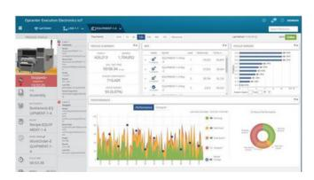
Opcenter Connect Electronics generates performance-based dashboards showing information by machine, line or factory level, including period summary, amount of pick-and-place errors, and general machine information.
