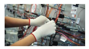
Wire harness manufacturing remains a labor-intensive process based on manual assembly.
