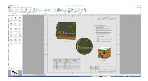
The **3D view** provides a virtual model of the assembled PCB. Customized 3D views of the PCB can be added to a sheet to enhance documentation.
